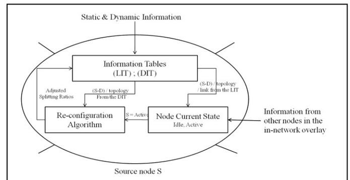
Figure 1. Components overview at the source node level
