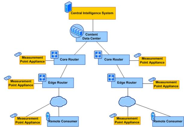
Fig. 1. Intra-domain perfSONAR deployment within a content-delivery network
