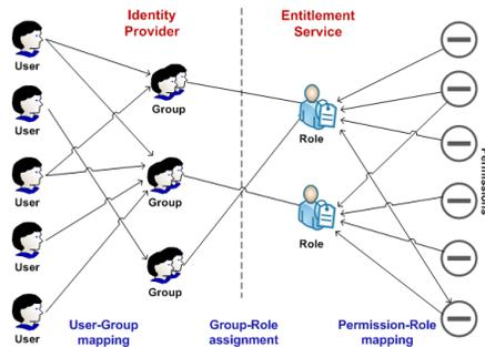
Fig. 4. Policy-engine design for user, group permission mapping
