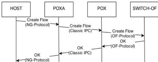
Fig. 3. Messages flow between Host and Switch-OF.
