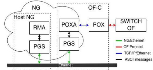
Fig. 4. Protocol stack inside and outside the NG cloud.
