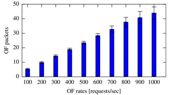
Fig. 7. Number of affected OF packets during migration process. The error bars indicate the standard deviation of the average values for all runs.
