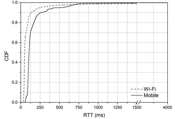
Fig. 8: RTT CDF for Wi-Fi and mobile networks
