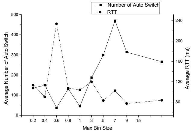
Fig. 6: Average number of auto switches and RTT for each bin size
