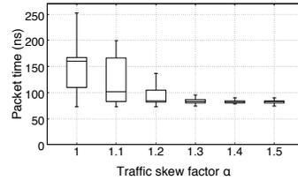
Fig. 1: Packet processing time vs. traffic skew
