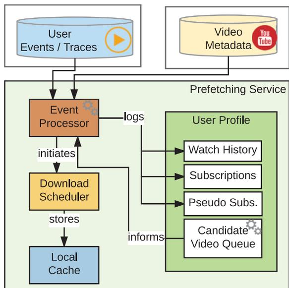
Fig. 8: Architecture of the vFetch Prefetching System
