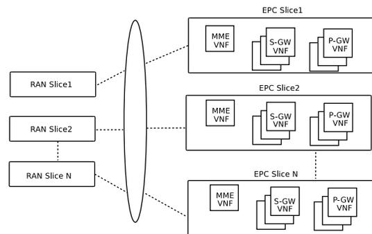
Fig. 2. Network Slicing System Model.
