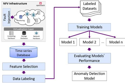
Fig. 2: Proposed ML-based anomaly detection method
