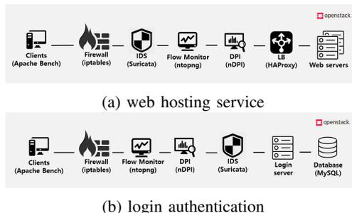
Fig. 4: Experimental testbed setup based on OpenStack: web hosting service scenario (a), login authentication scenario (b)
