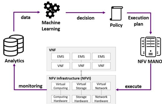
Fig. 1: Overall process of ML-based NFV management
