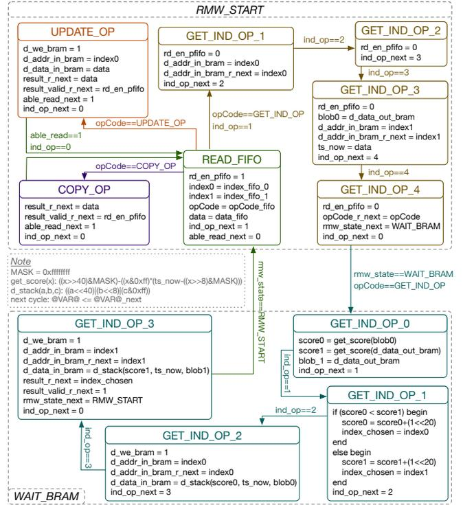
Figure 4. State machine in the dip\_reg\_score module.
