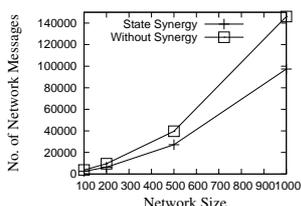
**Fig. 5.** Network messages are reduced with a state synergy (ave. -35%)
