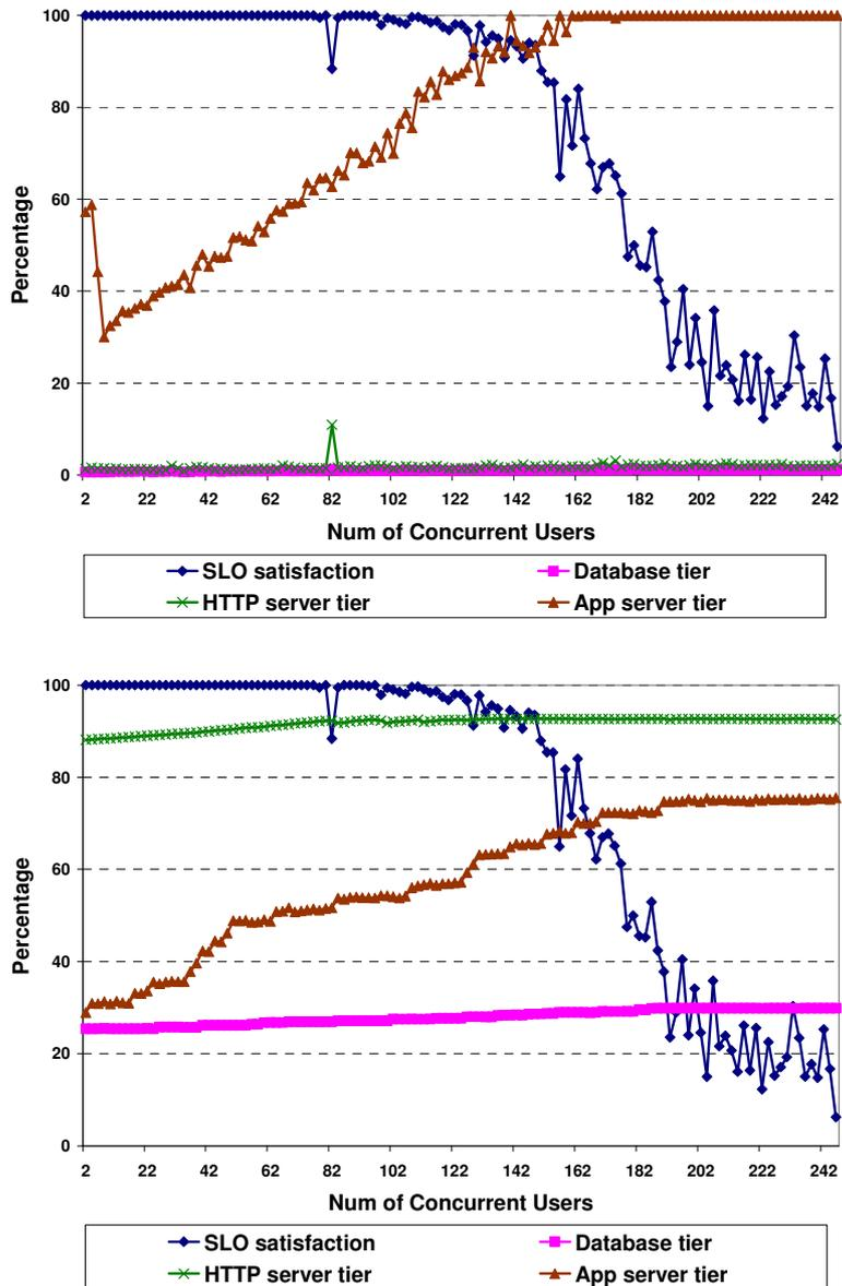
**Fig. 1.** SLO satisfaction against (a) CPU usage metric and (b) memory usage metric in all tiers.
