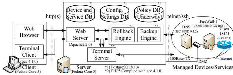
Fig. 2. Prototype Implementation Based on Proposed Scheme
