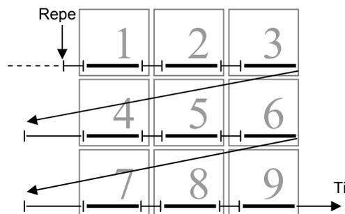
**Fig. 4.** Spatial-temporal mapping for vibro-tactile imaging:
