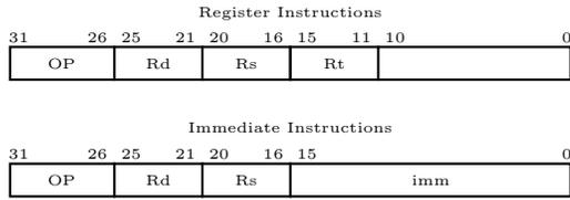
Fig. 1. Instruction set, Programmer’s Model, and Instruction Encoding
