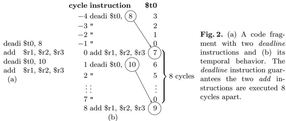
**Fig. 2.** (a) A code fragment with two *deadline* instructions and (b) its temporal behavior. The *deadline* instruction guarantees the two *add* instructions are executed 8 cycles apart.
