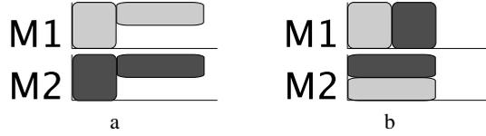
**Fig. 2.** By matching certain types of jobs, cooperative solution (b) delivers better makespans for both organizations than a solution scheduling all the jobs locally (a). The light gray jobs were produced by organization  $O_1$ , the dark gray ones by  $O_2$ .
