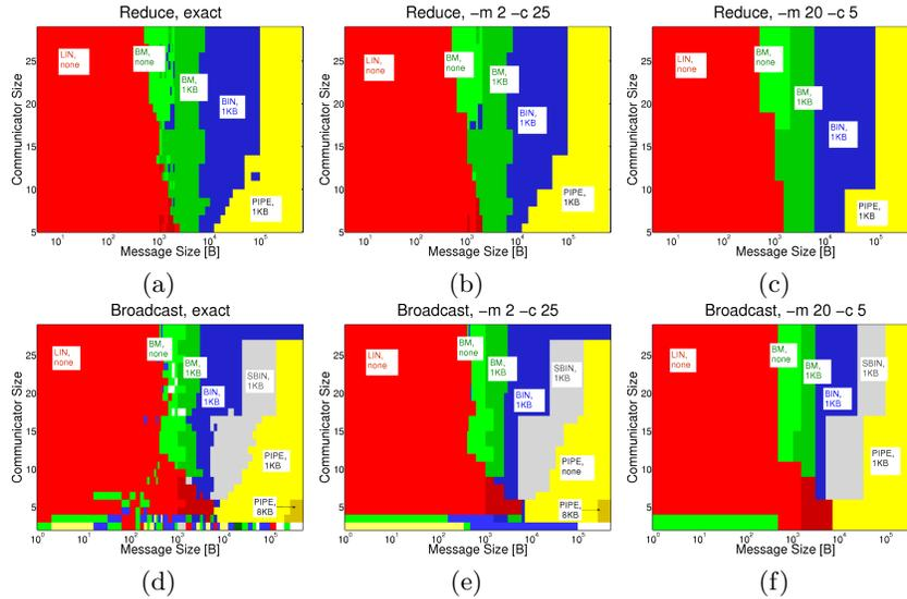
**Fig. 3.** Combined broadcast and reduce decision maps from the Grig cluster: (a) reduce, Exact (b) reduce, ‘-m 2 -c 25’ (c) reduce, ‘-m 20 -c 5’ (d) broadcast, Exact (e) broadcast, ‘-m 2 -c25’ (f) broadcast, ‘-m 20 -c 5’.
