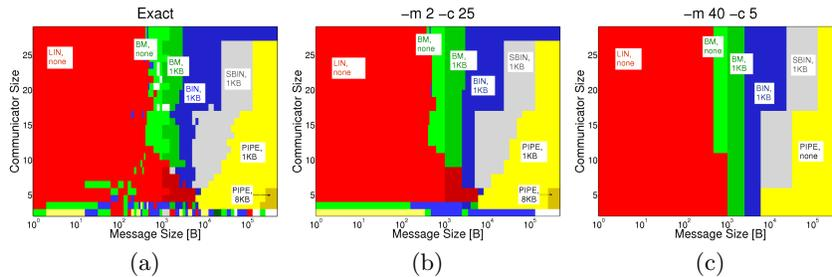
**Fig. 2.** Broadcast decision maps from the Grig cluster: (a) Measured (b)  $-m\ 2\ -c\ 25$  (c)  $-m\ 40\ -c\ 5$ . X-axis corresponds to message sizes, Y-axis represents the communicator sizes. Different colors correspond to different method indices. In this Figure, “LIN” stands for Linear, BM for Binomial, “BIN” for Binary, “SBIN” for Split Binary, and “PIPE” for Pipeline algorithm. Also, “none”, “1KB”, and “8KB” refer to the corresponding segment size.
