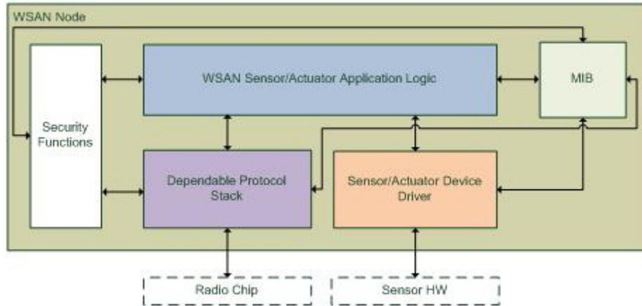
**Fig. 6.** Software architecture of the WSN node.
