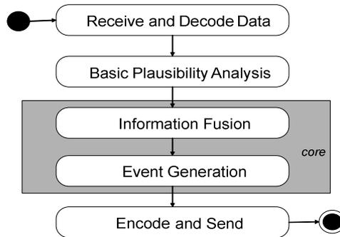
**Fig. 1.** Logical steps of the processing architecture
