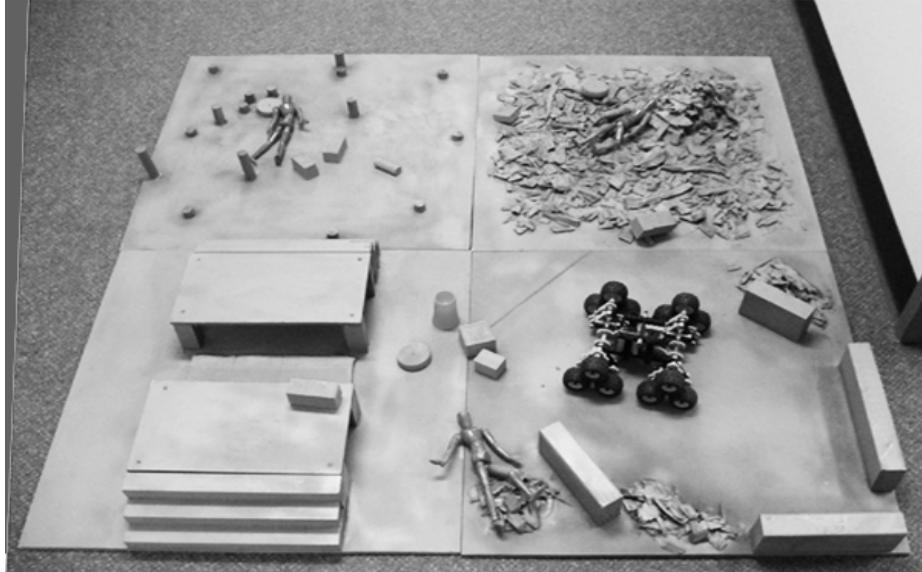
**Fig. 3.** 3-dimensional search and rescue robot arena. Four platform tiles arranged in a geomorphic configuration. The arena is populated with scaled-down effigies of victims, debris and moveable objects.
