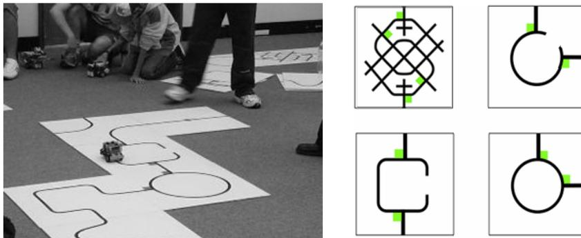
**Fig. 1.** 2-dimensional search and rescue robot arena based on RoboCup Jr (<http://www.robocup.org/>). Platform tiles are arranged edge-to-edge to provide a continuous path. Four samples from a possible pool of approximately 15 -18 different tiles are shown above. Tiles are designed with straight paths to increasingly complex paths.
