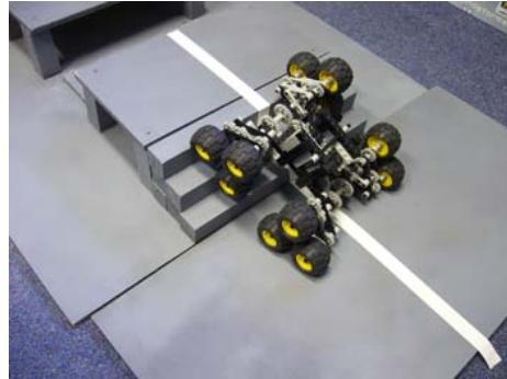
**Fig. 2.** 3-dimensional search and rescue robot arena. The entry-level category has a marked path to simplify the necessity to program complex navigational functionality into the scaled down SAR robots.
