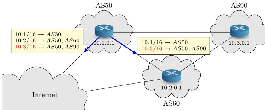
**Fig. 1.** Example of BGP prefix advertisement propagation. Two prefix advertisement messages sent from the router of Autonomous System AS50 are represented in the picture. AS50 is claiming to be able to reach the network 10.3.0.0/16 by being directly connected to AS90. AS60 and the other ASes on the Internet need to trust this piece of information from AS50.
