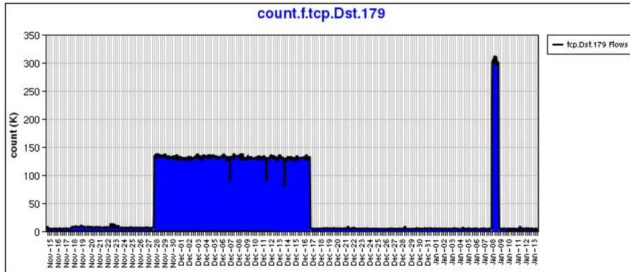
**Fig. 2.** Number of TCP flows per hour as detected by AT&T on their network (/8 prefix). The picture clearly marks two phases of our scanning activity at two different outgoing packet rates. It is noteworthy how scanning on port 179 is extremely more noisy than normal activity on that port.
