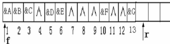
fig. 4 in order to store a binary tree after which is extended a complete binary tree
