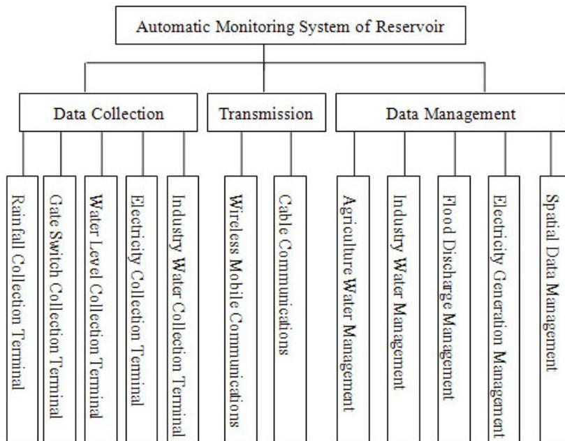
Figure 1. Structure of automatic monitoring system of reservoir
