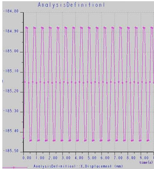
Fig.5 Horizontal displacement of the bottom shovel tip
