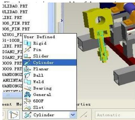
Fig.4 Linking constraint assembly of the experiment-table
