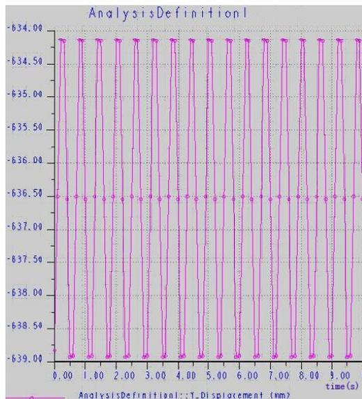
Fig.6 Vertical displacement of the bottom shovel tip
