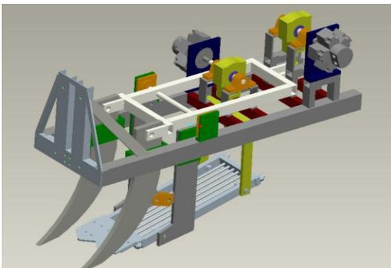
Fig.2 The digital element model of the 1WZ-type deep rhizome crops excavating test-bed
