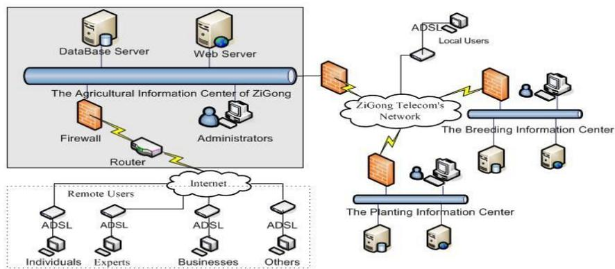
Fig 1. The Network Structure
