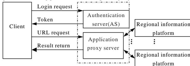
Fig. 3. SSO system architecture
