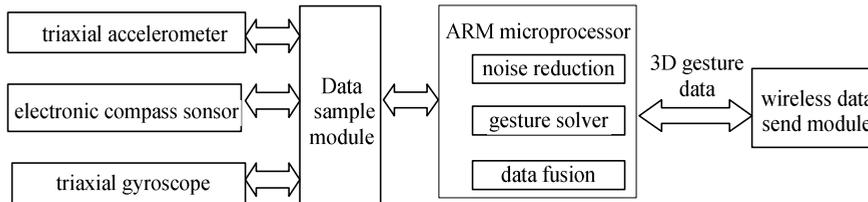
**Fig. 3.** The arm gesture detection module hardware frame
