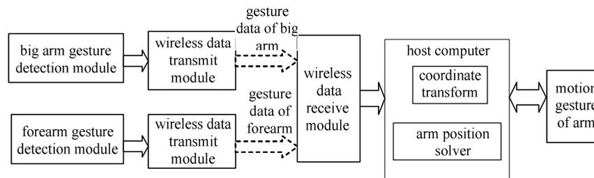
**Fig. 2.** The arm movement track system hardware frame
