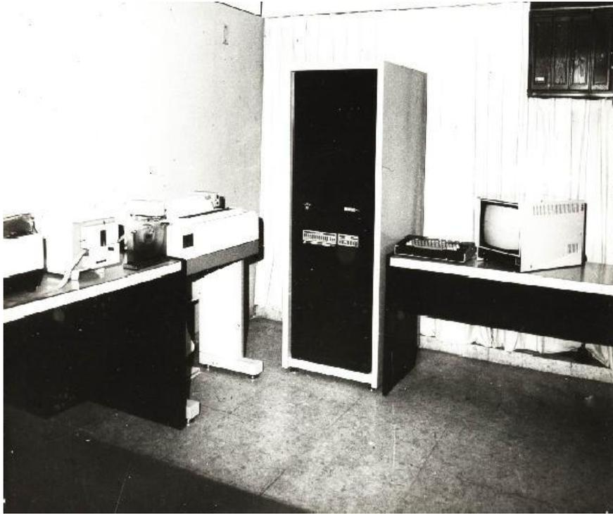
**Figure 3** Cuban minicomputer system CID 300/10.
