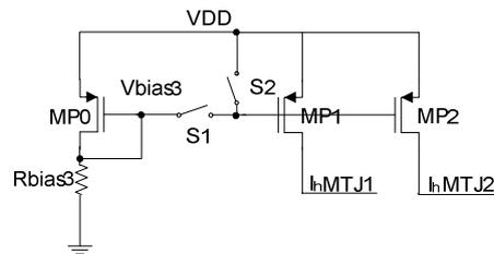
Fig. 7. Unidirectional current generator.
