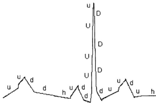
**Fig. 1** - Piecewise linear approximation of an ECG signal [12]
