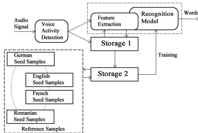
**Fig. 1.** The general structure of our system showcasing the main modules and data flow between them and the seed samples needed for clustering into phonetic clusters. As well as the separation between the recognition process, the acquisition process and the reference samples needed for clustering.
