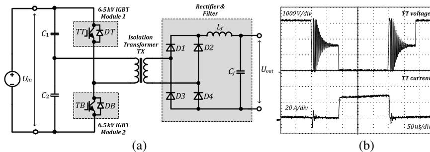
**Fig. 1.** Hard-switched high-voltage half-bridge converter topology (a) and measured IGBT voltage and current waveforms (b).
