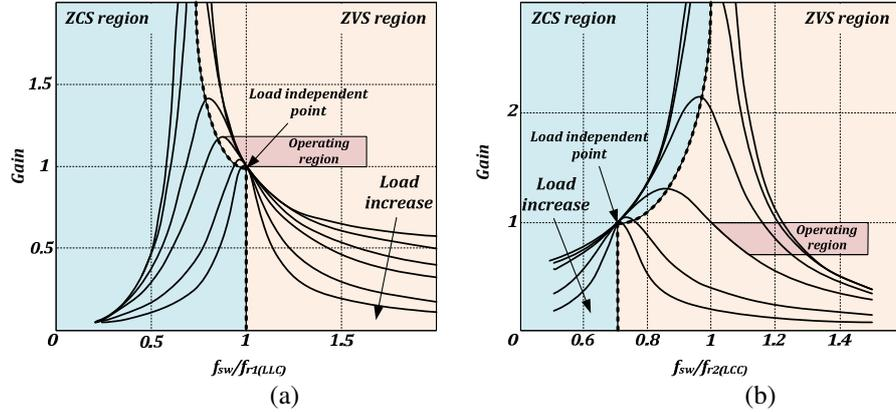
**Fig. 3.** Generalised voltage gain vs. normalised frequency at different loads for LLC converter (a) and LCC converter (b).
