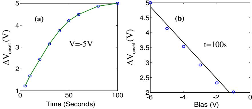
**Fig. 6.** (a) Change in onset voltage as function of time when a reverse voltage (-5V) is applied; (b) change in onset voltage for increasing reverse bias measured with a fixed time duration ( $t=100s$ )
