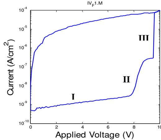
**Fig. 3.** Typical current-voltage characteristics during electroforming of Al/Al<sub>2</sub>O<sub>3</sub>/polyspirofluorene/Ba/Al diode
