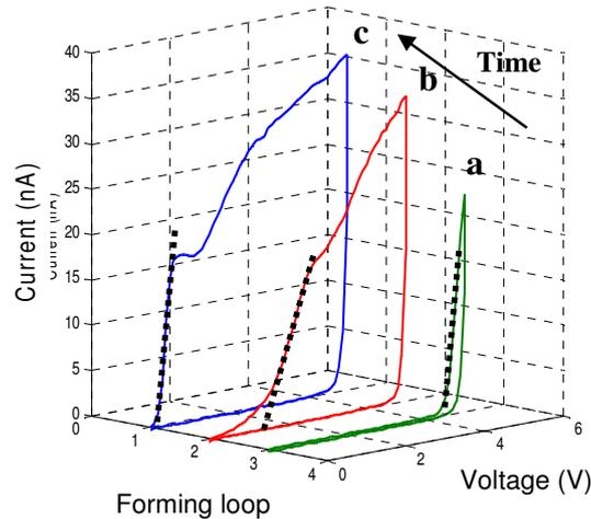
**Fig. 4.** Time dependence of the electroforming loops. A device electroformed to 5V will approximately have the onset voltage of 5V (*curve (a)*). By leaving the device resting in dark, the forming loop (*a*) will evolve to curve (*b*) and eventually (*c*). The onset voltage estimated by the intercept with the voltage axis (*dash line*) will decrease with time to below 1V
