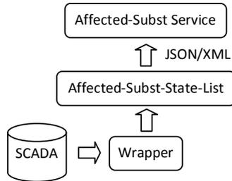
Fig. 4. Distributor's service integration for substation incident triggers.
