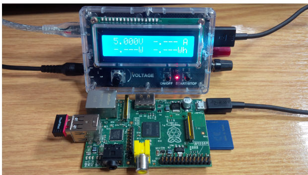
Fig. 1. Odroid smart power measurement tool
