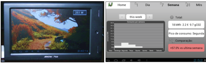
Fig. 3. Different views from the WattsBurning system. Left: Forest visualization of the electricity consumption. Right: Graphical representation of the weeks consumption.
