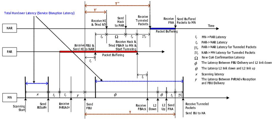
**Fig. 1.** Origin FMIPv6 handover procedure and timing diagram in case of receiving FBACk via the previous link
