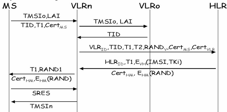
Fig. 2. Secure TMSI Allocation Procedure
