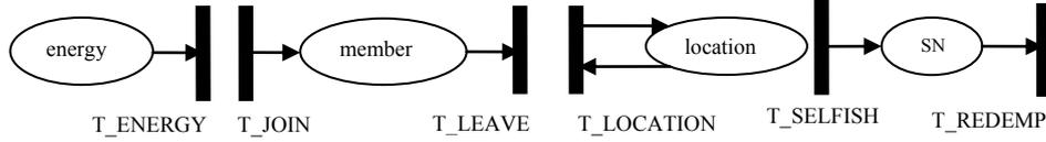
**Fig. 2.** SPN subnet for describing the status of a node.
