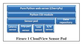
sensors. It provides the web service interface which is invoked by CloudView information manager. It also provides scheduling and invocation services for taking instant (non-scheduled measurements requested by the user in real-time) and periodic (repeating measurements scheduled in advance) measurements. The data repository stores the measurement data collected by sensors in periodic measurements for later retrieval.
