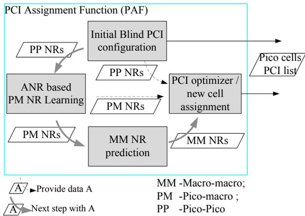
Fig. 4. The PCI Assignment Function (PAF)
