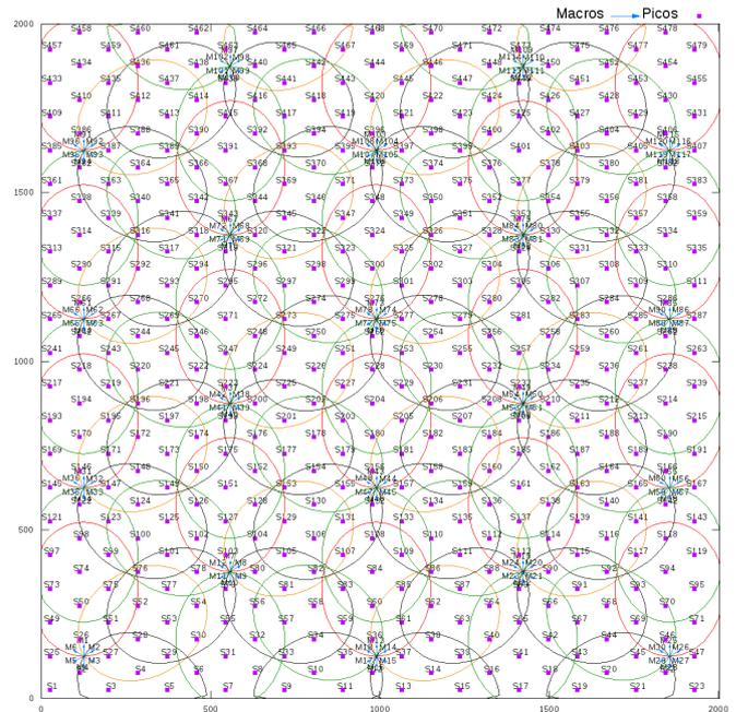
Fig. 9. Example UDN model: 6-sector macro sites with 500 m ISD and omnidirectional pico cells with 100 m ISD
