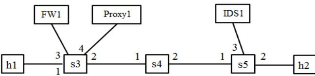
Fig. 4. Experimental physical topology
