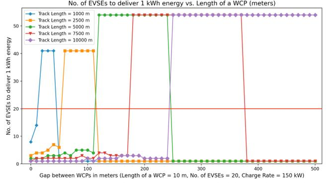
Figure 7: Gap between WCPs in meters vs. No. of EVSEs to deliver 1 kWh energy.
