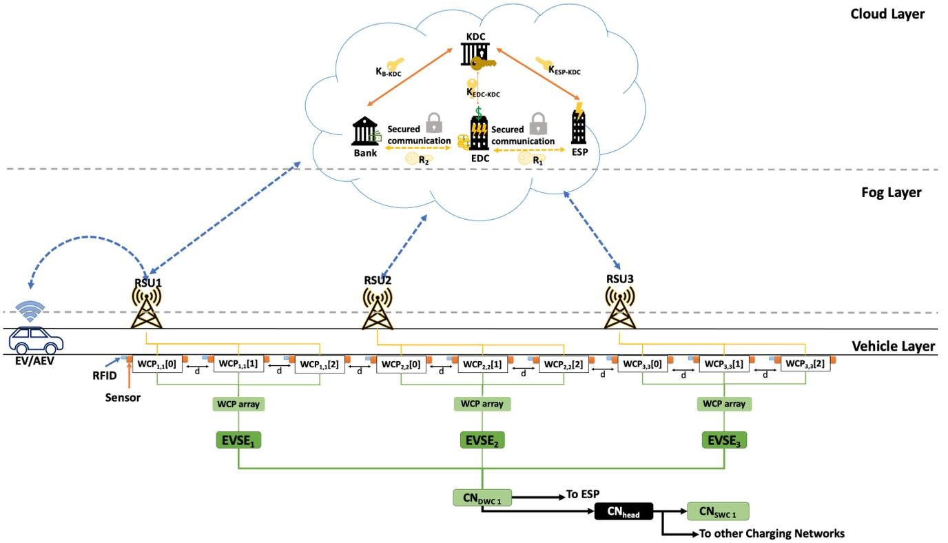
Figure 2: DWCN following the proposed three-layer hierarchical design.
