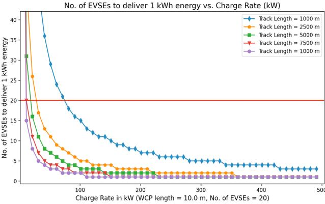
Figure 4: Charge rate in kW vs. No. of EVSEs to deliver 1 kWh energy.
