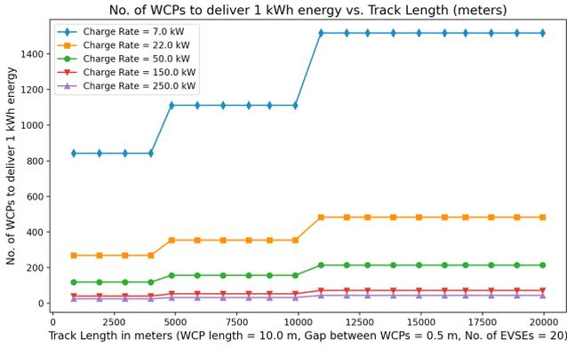
Figure 3: Track length in meters vs. No. of WCPs to deliver 1 kWh energy.
