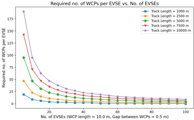
Figure 5: No. of EVSEs vs. Required no. of WCPs per EVSE.
