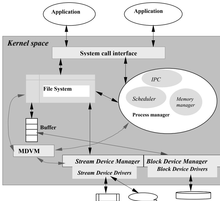
Figure 3. MDVM System within a Monolithic Kernel.
