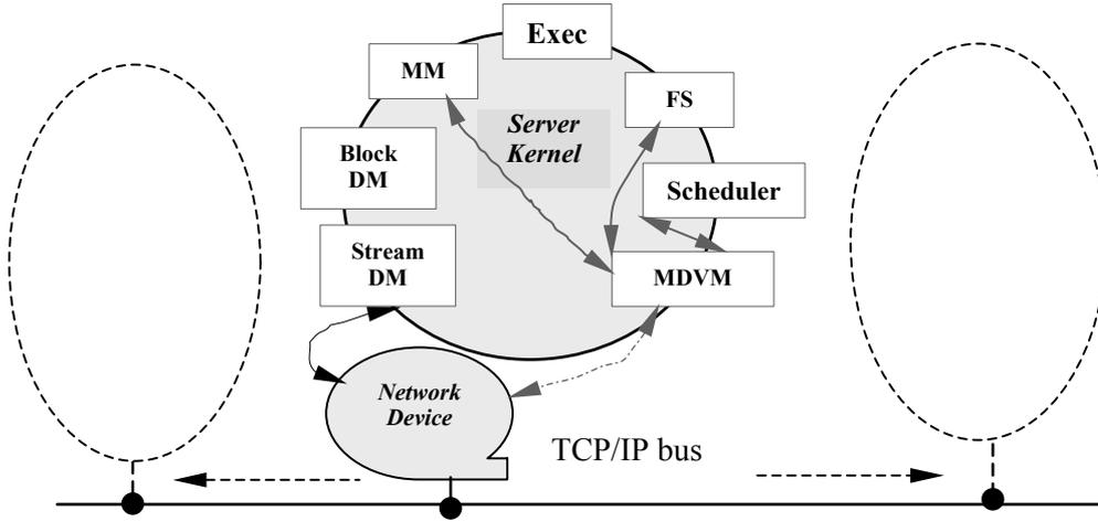
Figure 5. Interfaces between MDVM Device and Monolithic Kernel Subsystems.
