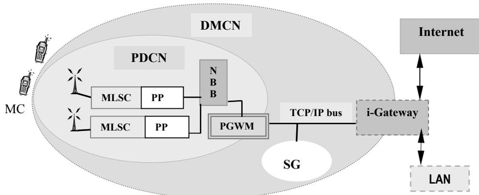
PDCN: Packet Data Communication Network, MLSC: Mobile Local Switch Center, PP: Packet Processor, NBB: Network Backbone, PGWM: Packet Gateway Module.
