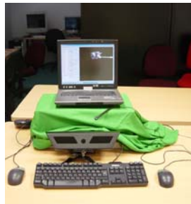
Fig 3. Set-up for the usability study (including a third mouse for the leader of the experiment to start and stop applications)
