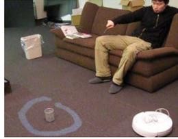
**Fig. 8.** Visual Feedback on Laser Trajectory
