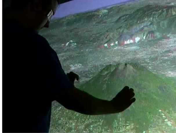
**Fig. 1:** A user interacting with an interscopic multi-touch surface (iMUTS) in a landscape planning scenario in which depth cues are important, e. g., in a landslide risk management scenario. The geospatial data is displayed in anaglyph stereoscopic mode.
