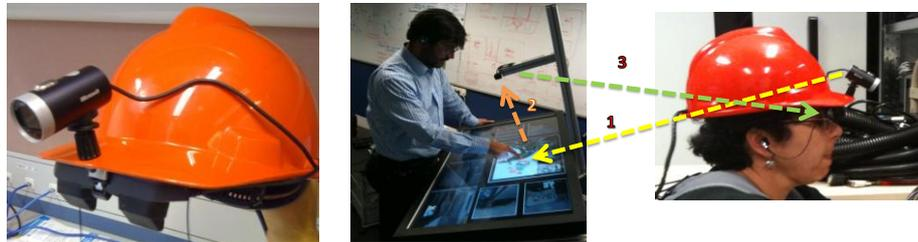
**Fig. 1** Left: helmet with camera and near-eye display. Right: system work flow.
