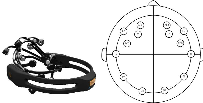
**Fig. 1.** A low-cost EEG device (Emotiv EPOC neuroheadset [10]) and layout of EEG channels.
