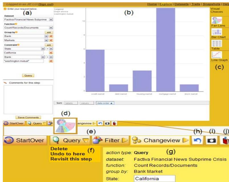
**Fig. 1.** Smarter Decisions user interface: (a) query panel, (b) visualization canvas, (c) alternate visualization choices, (d) thumbnail of the visualization for a step, (e) trail steps, (f) menu of operations for a step, (g) detail of the action performed during a step, (h) undo, (i) snapshot, (j) bookmark.
