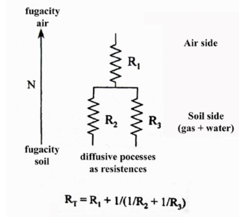
Fig. 1. Three resistance concept based on fugacity approach [10].
